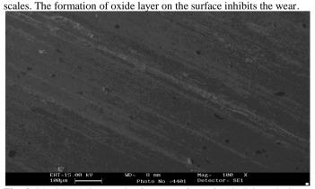
**Fig. 2 (a):** SEM Micrograph of worn surface of AISI D3 steel pin at speed 1.15 m/s
