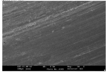
**Fig. 2(c):** SEM Micrograph of worn surface of AISI D3 steel pin at speed 2.56 m/s
