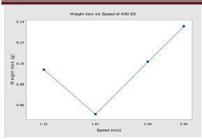
Fig. 1(a): Friction behaviour of AISI D3
